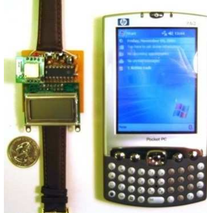
Fig. 6. The prototype of a watch as the interface cache for iPAQ
