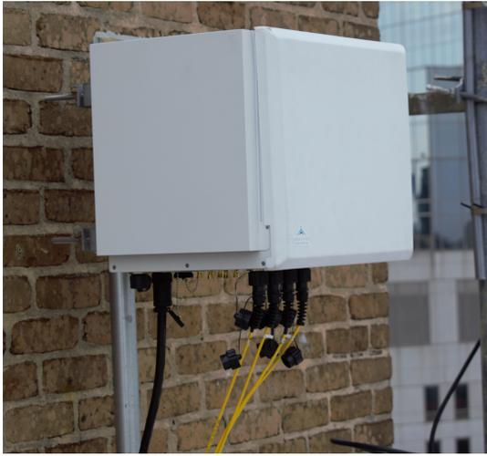
Fig. 1. Single 160-radio CBRS weatherproof ArgosV3 base station mounted outdoors. Four single-mode fiber pairs provide up to 40 Gbps connectivity.
