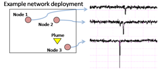
Figure 10: A demonstration deployment of 3-node real-time wireless sensor network measuring an O 2 plume. Data is synchronized and acquired continuously, and the plume could be localized using time-of-flight with nodes ~3 meters apart. The concentration signal is inverted due to the selected phase of the lock-in.
