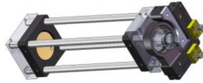
Figure 9: 31 pass multipass cell model in Solidworks designed from mostly off-the-shelf parts.
