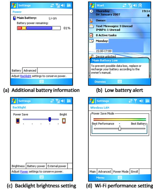
Figure 2. Battery interfaces on the HTC Wizard phone
