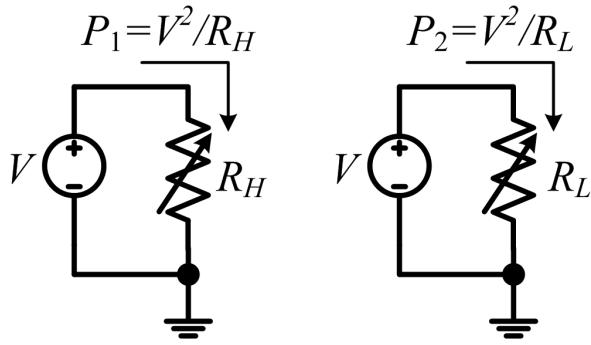
Figure 6. The power consumption of accessing a device in HR state ( $R_H$ ) and a device in LR state ( $R_L$ ) is  $P_1$  and  $P_2$ , respectively. When  $R_H / R_L$  is high enough, the difference between  $P_1$  and  $P_2$  will be significant.
