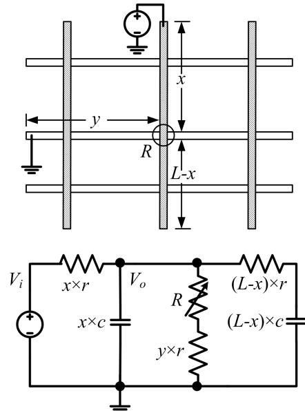
Figure 5. Equivalent circuit of a crossbar memory, where  $L$  is the length of a wire,  $r$  is unit resistance of a wire,  $c$  is unit capacitance of a wire. The delay to access the device with solid circle is affected not only by the position ( $x$ ,  $y$ ), but also by the content ( $R$ ) of the device.
