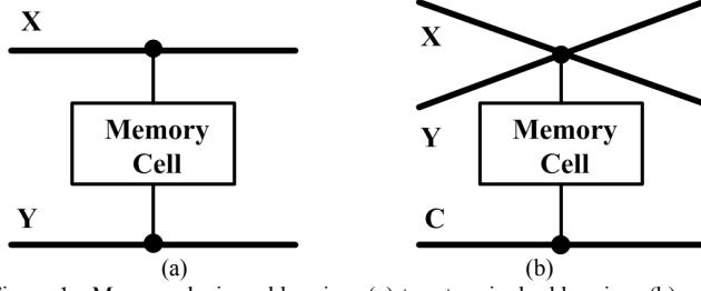
Figure 1. Memory device addressing; (a) two-terminal addressing; (b) one-terminal addressing.
