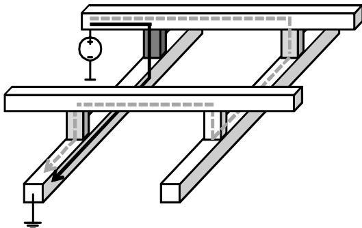
Figure 3. Two-terminal addressing does not function correctly in a  $2 \times 2$  crossbar of symmetric memory devices. Because the white device is symmetric, an extra current (the grey dashed arrow) will interfere the current we need to sense (the black solid arrow) and we will get a wrong content of the dark grey device.
