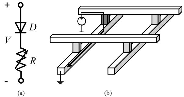
Figure 2. (a) A two-terminal asymmetric memory device; (b) A  $2 \times 2$  crossbar of asymmetric memory devices. By applying a voltage and sensing the current (the black solid arrow), we can read out the information stored in the dark grey device.
