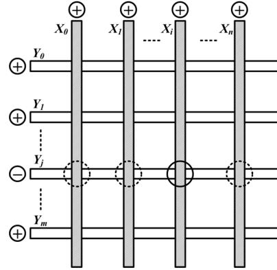
Figure 4. Proper voltage assignment (positive: voltage source; negative: ground) makes a crossbar with symmetric memory devices function correctly. By sensing the current flowing from  $X_i$  to  $Y_j$  at the terminal  $X_i$ , we can read out the information stored in the device with the solid circle. There also exist other currents such as the one from  $X_0$  to  $Y_j$  and the one from  $X_i$  to  $Y_0$ , which will lead to not an error but a significant energy waste.
